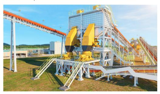
A dozen of core technologies for green and smart mines such as pebble crushing by High Pressure Grinding Roll (HPGR) to provide green solutions for metal and non-metal mines in different sizes
